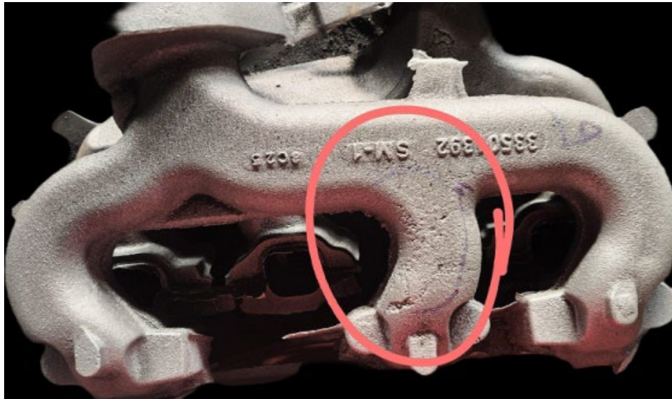
Fig. 4 Sand drop defect of Manifold
