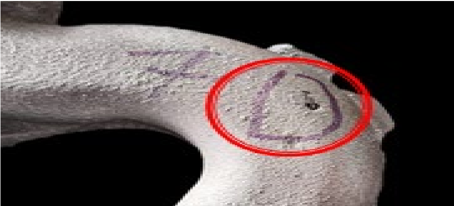
Fig.6 Blow hole defect in Manifold
