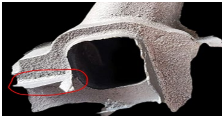
Fig.10 Shift defect in manifold
