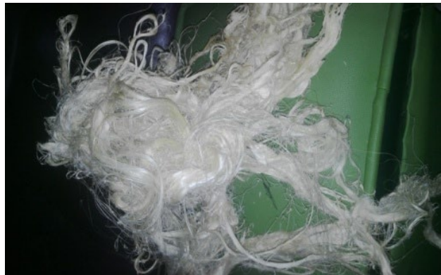
Fig. 3 Extracted Sisal fibre
