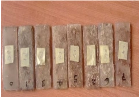
Fig. 6 Flexural test samples
