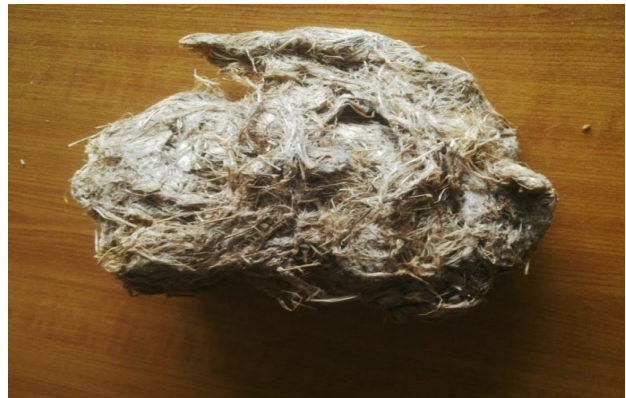
Fig. 4 Extracted Plantain fibre.
