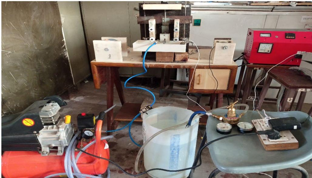
Fig. 3 Mist flow aided WECDM setup
