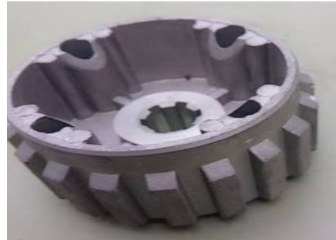
Fig. 10 CY 80 motorcycle clutch hub after machining and finishing
