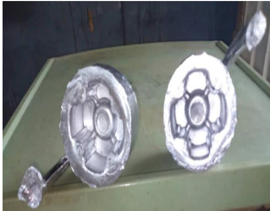
Fig. 9 The CY80 motorcycle Clutch Hub before machining and finishing
