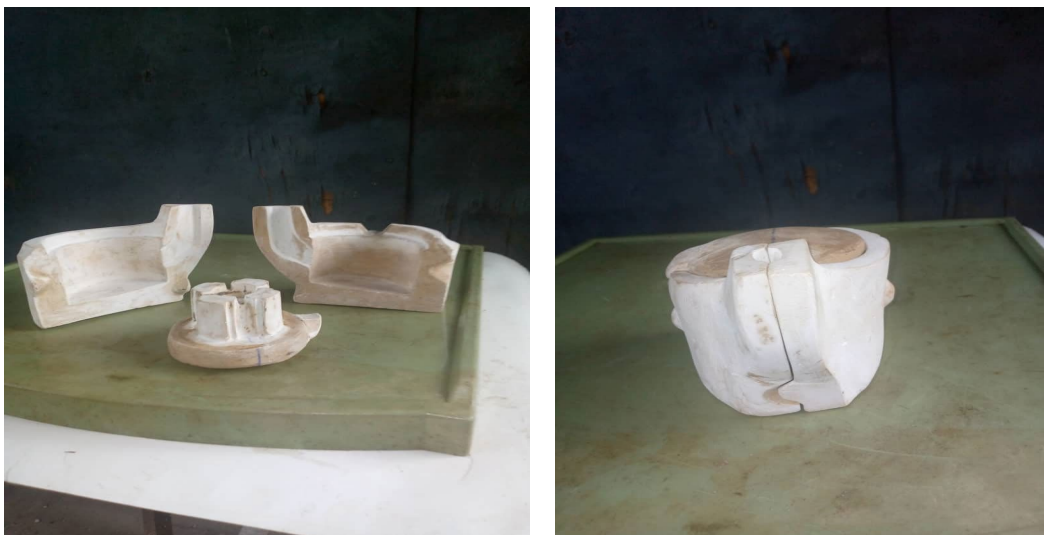
Fig. 3 The pattern and core for the clutch hub mould
