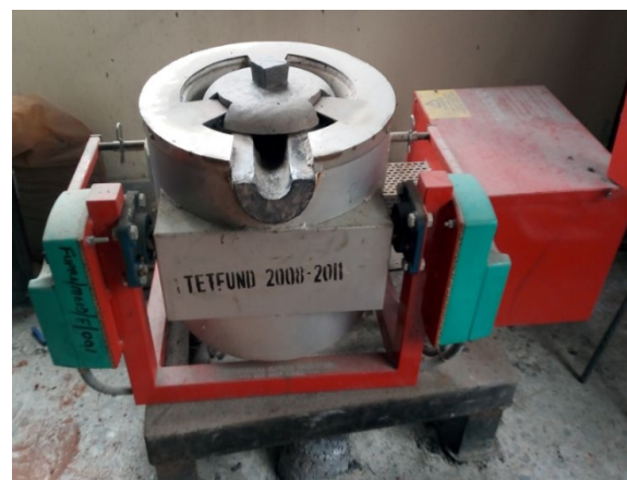
Fig. 5 Electrically operated gas crucible furnace
