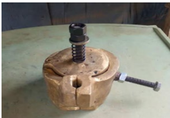
Fig. 4 The permanent mould made from brass for the clutch hub
