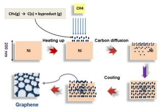
Fig. 2 Mechanism of CVD method on Ni substrate [23]
