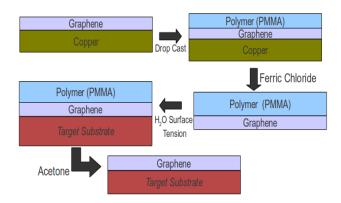
Fig. 3 Schematic diagram of the transfer process [25]
