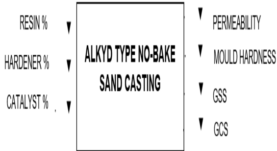
Fig. 1 Input-output model for Alkyd type no-bake sand casting process
