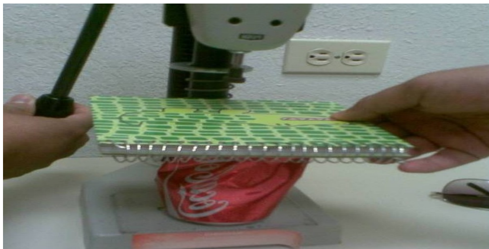
Fig.4 Dynamometer Used to Crush a Single Can Organized Vertically
