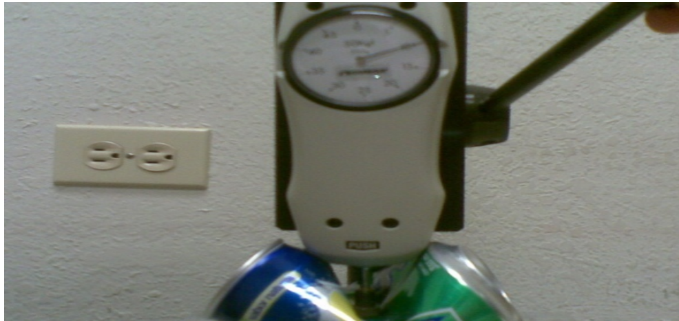
Fig.3 Dynamometer Used to Crush a Single Can Organized Horizontally
