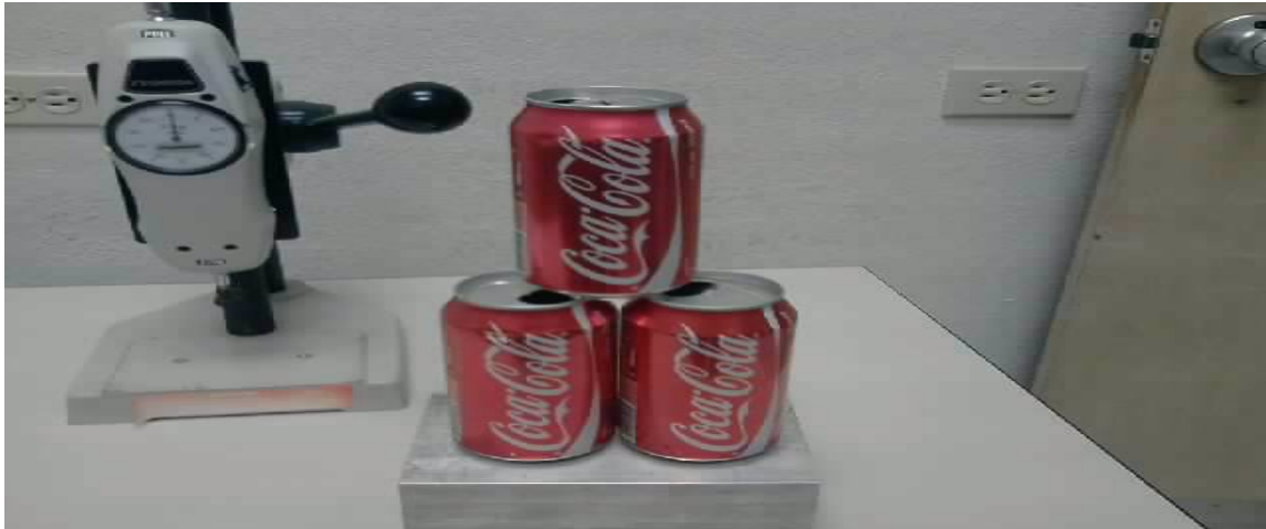
Fig.1 Dynamometer Used to Crush three Cans a Time Organized as Shown
