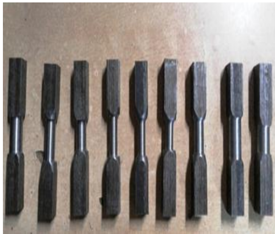
Fig. 1 Mild steel hollow specimens
