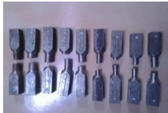
Fig. 2 Specimens after Torsion failure
