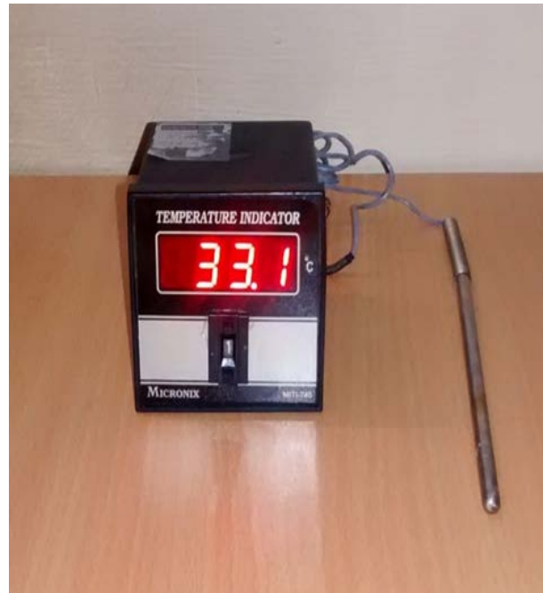
Fig. 8 Digital temperature indicator with RTD PT100 Sensor
