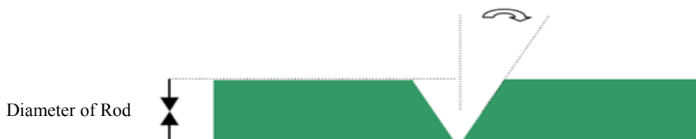
Fig. 1 Stainless Steel specimen with single v groove
