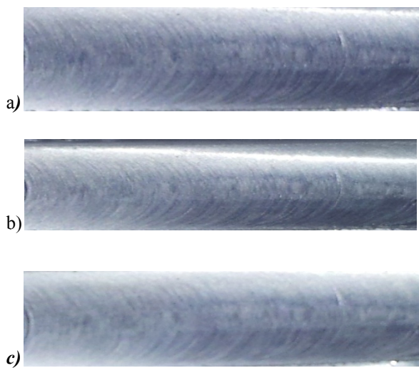
Fig. 3 Macrographs of specimens processed with FSP under natural cooling condition with different tool-pin profiles (a) square tool, (b) hexagonal tool, (c) round tool.
