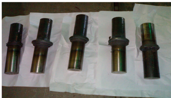
Fig. 1 Shows friction welded samples
